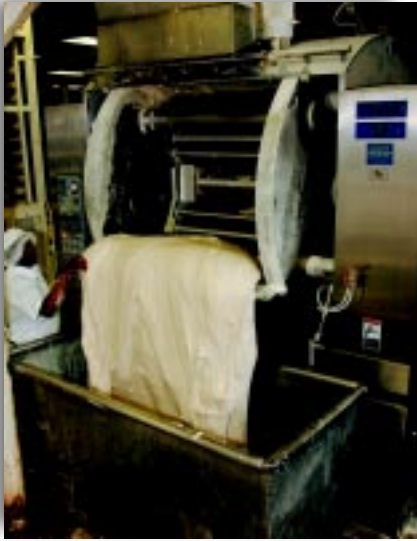
◀ The bakery utilizes the latest technologies such as this Peerless final mixer with Cold Bar temperature control.
