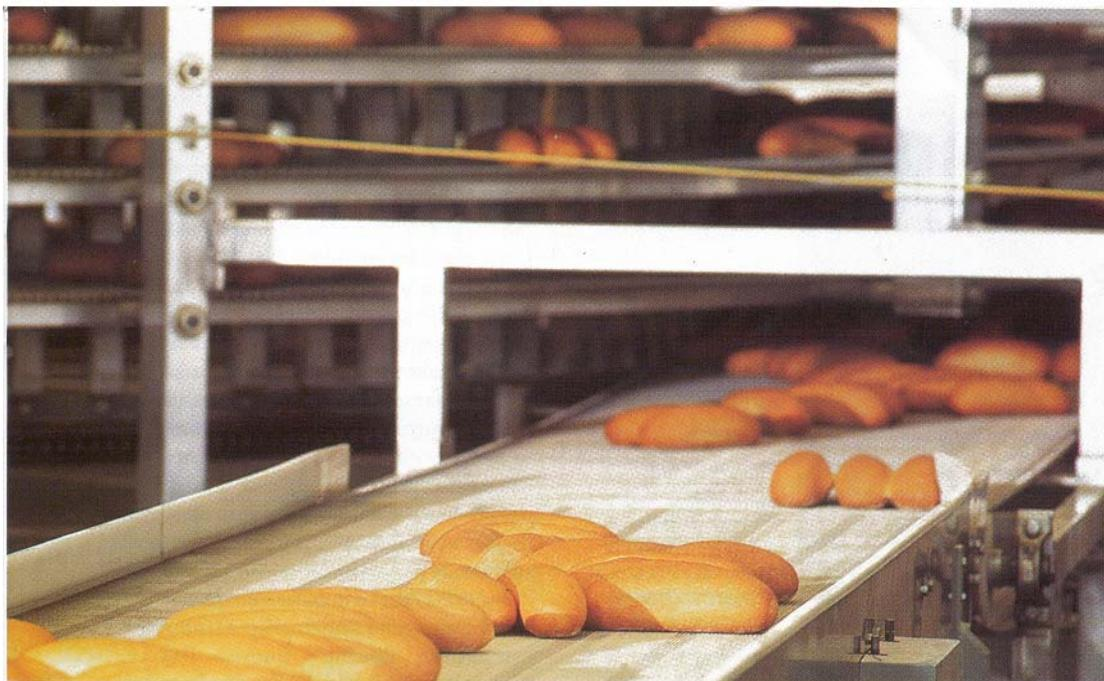
The spiral conveyer installed between the oven line and the packaging room assures rapid, uniform cooling while minimizing handling.
